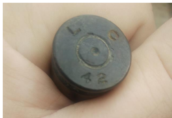
Figure 8. .50 calibre case found at wreck site, the primer has been struck indicating the round was fired prior to the crash. The markings indicate the factory of manufacture and the date, in this case Lake City Army Ammunition Plant, Missouri 1942. Photo by author.
